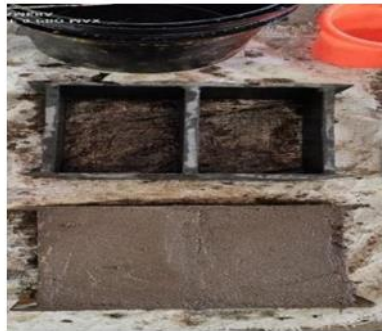
Placing of mixed materials in mould
