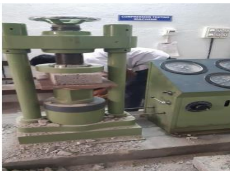
Figure 4: Compressive Strength test
