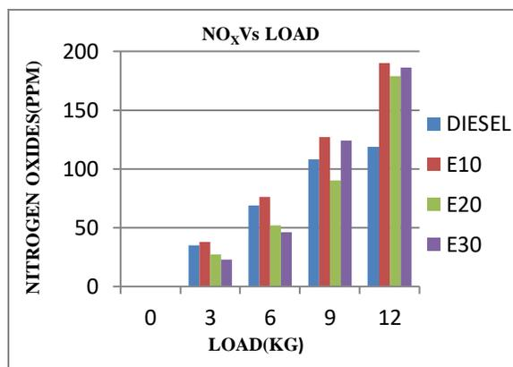
Figure 8: Oxides of Nitrogen Vs Load
