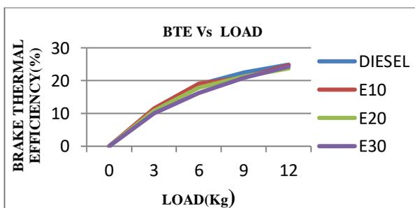
Figure 4: Brake Thermal Efficiency Vs Load
