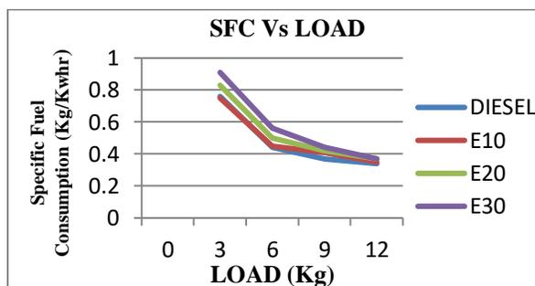
Figure 3: Specific Fuel Consumption Vs Load
