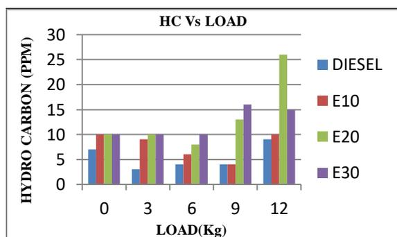
Figure 6: Hydro carbon Vs Load
