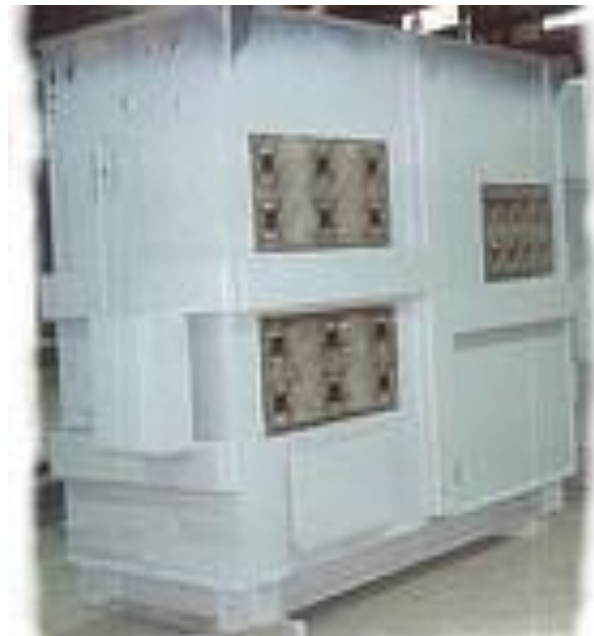
Figure 3: Body of transformer
