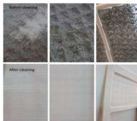
Figure 1: The accumulated dust that contains the microorganism on discarded polyester filters before and after cleaning (Al-Abdalla et al. , 2019).
