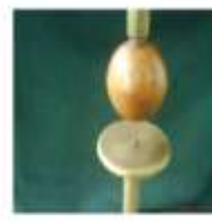
(b) Sphere-Plane Configuration
