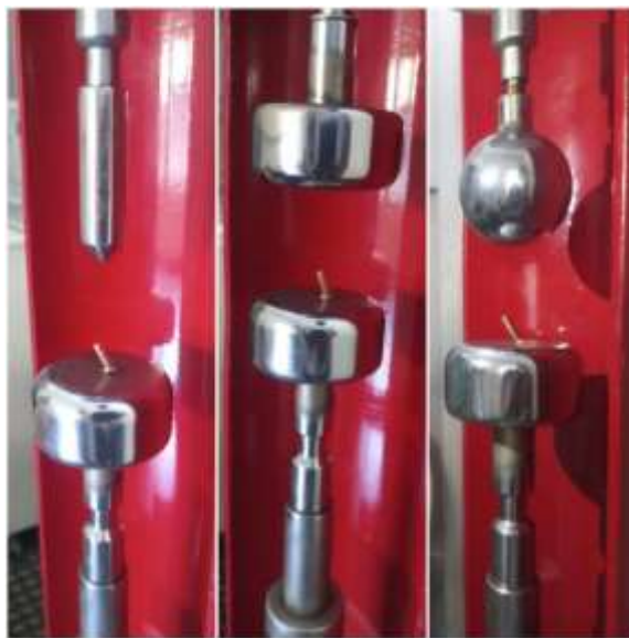
Figure 4: Electrode configurations used for the experiment
