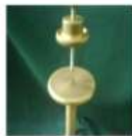
(c) Rod-Plane Configuration
