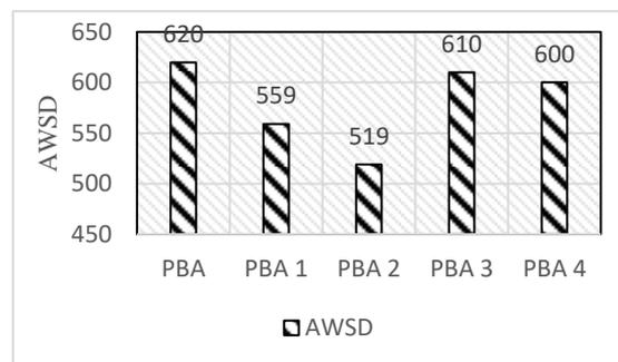
Figure 3: AWSD of formulated nano lubricant
