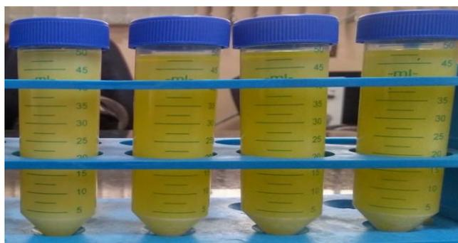
**Figure 1:** Bitter almond oil-based nano-lubricant (PBA1, PBA2, PBA3, PBA4 L to R)
