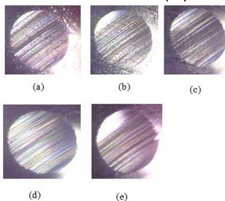
Figure 4 Optical microscopic images of worn-out surfaces of balls under formulated nano lubricant (a) PBA (b) PBA1 (c) PBA2 (d) PBA3 (e) PBA4
