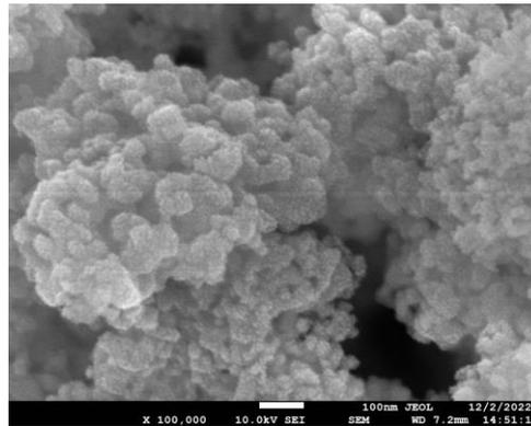
Figure 2: FESEM image of TiO<sub>2</sub> nanoparticles
