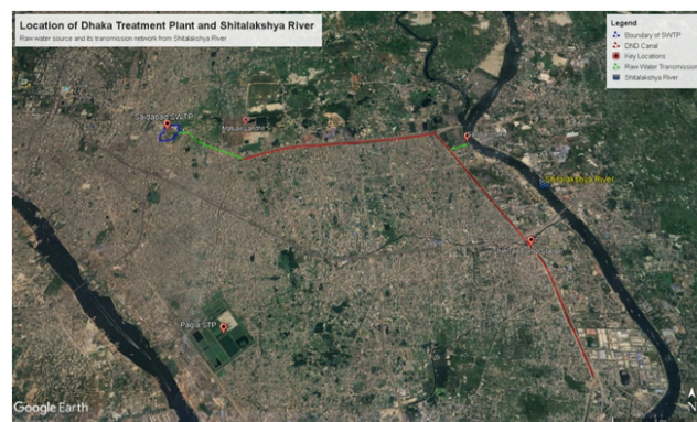
Figure 1: Raw water source and its transmission network from Sitalakhya River to WTP
