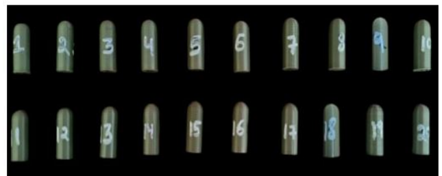
Figure 1(b): ASTM standard 3-D printed wear test samples at various input parameters setting
