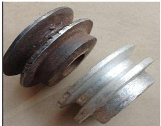
Figure 13: Steel and Hybridized Pulley
