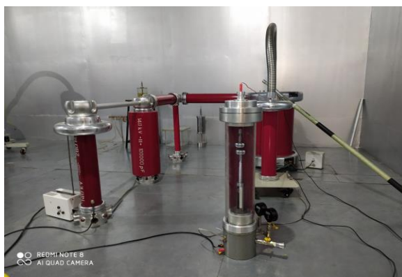
Figure 2: Laboratory setup for breakdown voltage measurement
